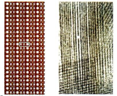
**Figure 2.** Ordered intergrowth structural model (left) and HREM image of synthesized material with disordered intergrowth (right) (TEM photo by Charles Bateman).
